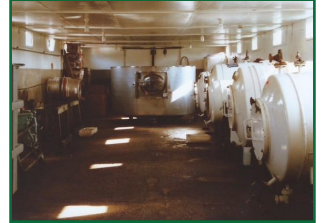
1980. The Fermenting Room (mid-late 1980). Of note is the Yorkshire Square-style fermenting vessel on the left, the yeast press beyond and the horizontal conditioning tanks along the right.
